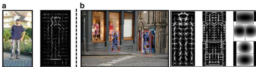
**Fig. 1** (a) A sample positive image and its HOG descriptor. (b) *Left*: detections obtained using part-based human detector in [6]. *Right*: a model for root and parts and a spatial model for the location of each part relative to the root
