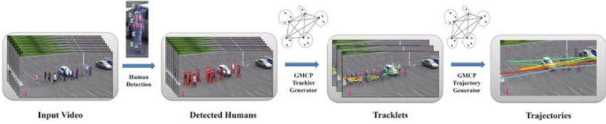
**Fig. 3** Block diagram of the data association method. A video is divided into smaller segments, and the GMCP-based method is employed to find pedestrian tracklets and trajectories
