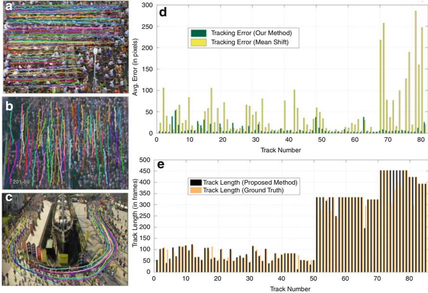
**Fig. 9** (a–c) Tracked individuals in the three sequences. (d) Comparison with Meanshift. (e) Comparison with ground truth
